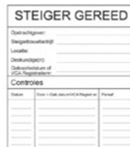
Completed scaffold tag in the tag holder, as soon as scaffold is completed
